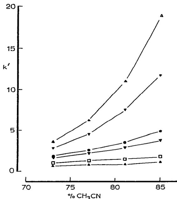
Fig. 2. Effect of eluent acetonitrile content upon  $k'$  of a standard polyol-saccharide mixture.  $\Delta$  = Trehalose;  $\nabla$  = sucrose;  $\bullet$  = sorbitol;  $\nabla$  = fructose;  $\square$  = erythritol;  $\blacktriangle$  = glycerol. Other conditions as in Fig. 1.
